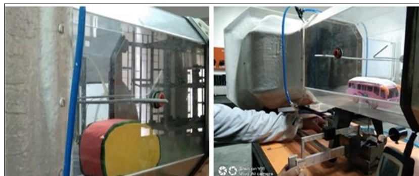
Fig 5: Setup in experimental wind tunnel for base model modified-1 & 2
