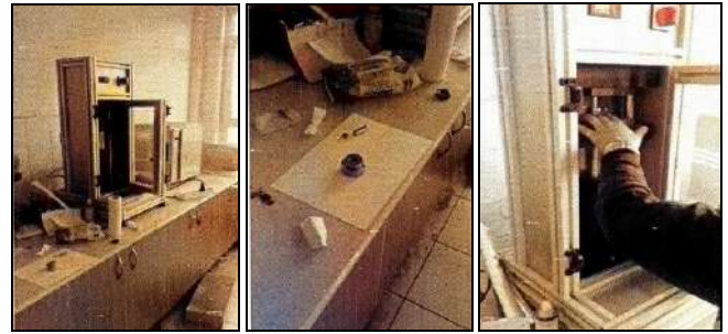
Fig 4: Mold material, pressing machine and placing the mixture placed in the mold in the machine for the process
