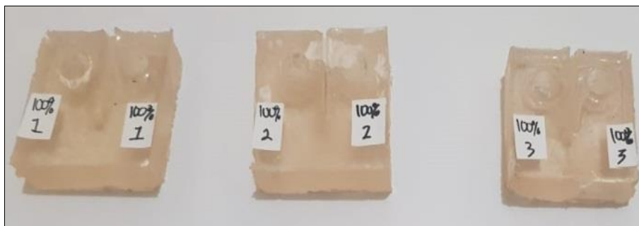
Fig 2: Example of casting result from crack test sample according to ASTM D5405.
