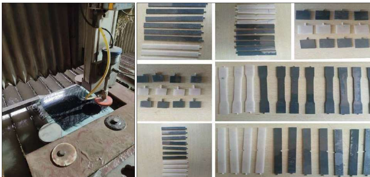
Fig 3: Machining of laminate & specimens as per standards
