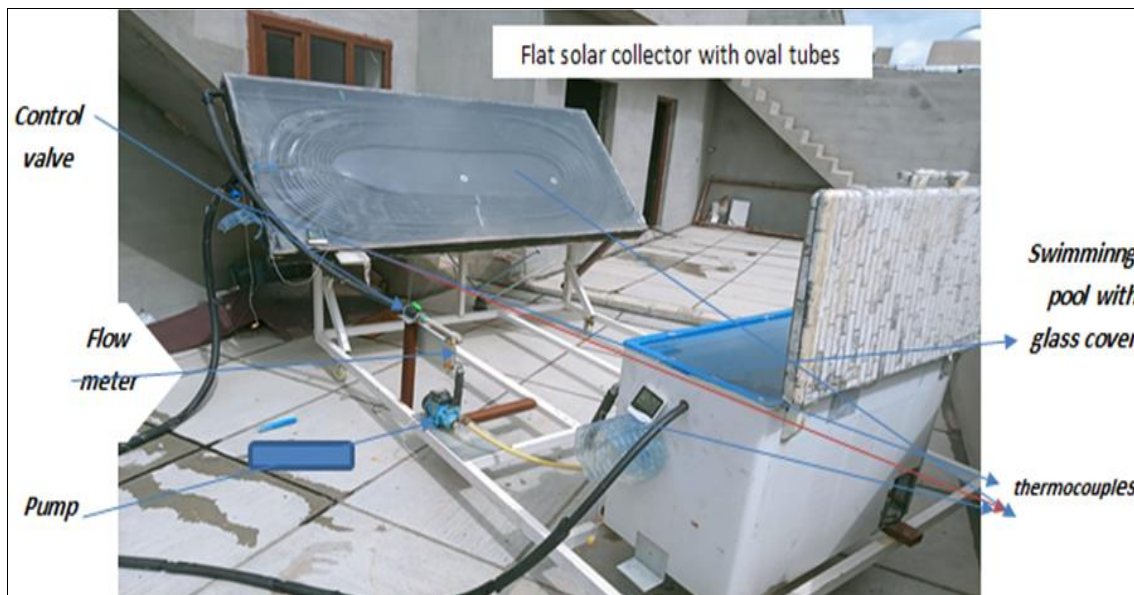
Fig 1: Solar collector with swimming pool and accessories
