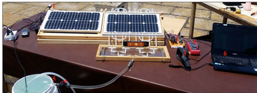
Fig 7: (1) Solarimeter, (2) Control board, (3) Thermal camera, (4) Thermocouple, (5) water pumping system, (6) Computer for recording Data.
