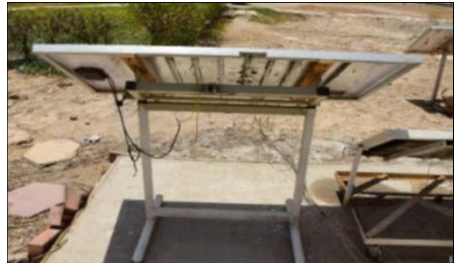
Fig 5: PV-Aluminium Finned Wall module structure.
