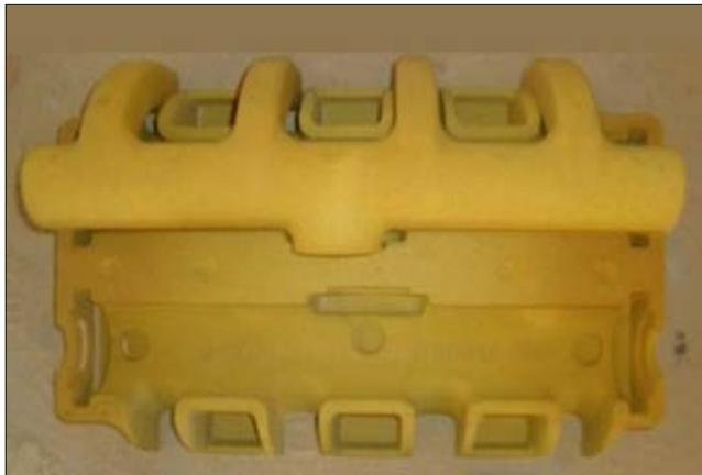
Fig 1: Moulding from resin coated sand
