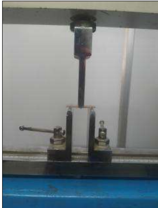
Fig 3: Bending test of sample
