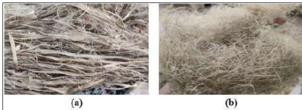
Fig 1: (a) Un-carded fiber, (b) Carded Fiber
