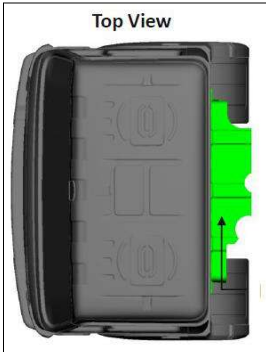
Fig 4(a): Horizontal deflector
