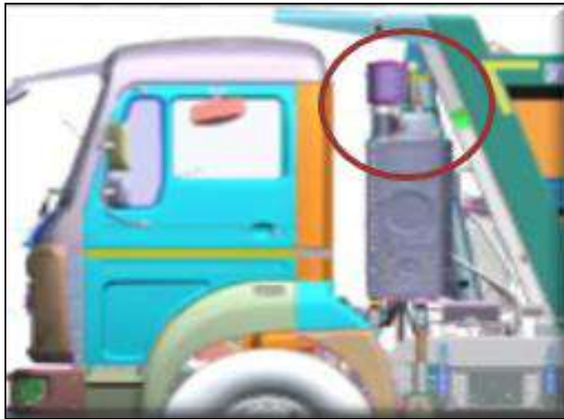
Fig 2(a): Base configuration with box type diffuser
