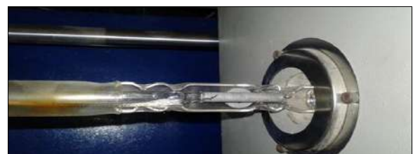
Fig 16: Dilatometer tube with specimen
