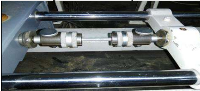
Fig 22: Tensile test broken specimen
