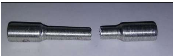
Fig 13: Tested specimen (broke at right side)
