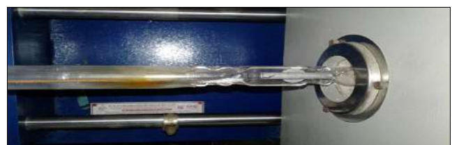
Fig 25: Specimen placed in glass tube
