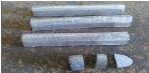
Fig 2: Aluminium-strontium super alloy ingot of 10% Sr
