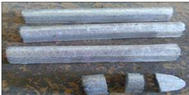
Fig 3: Aluminium-strontium super alloy
