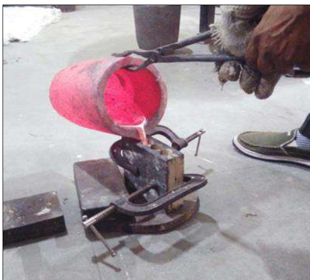
Fig 10: Pouring of molten metal into
