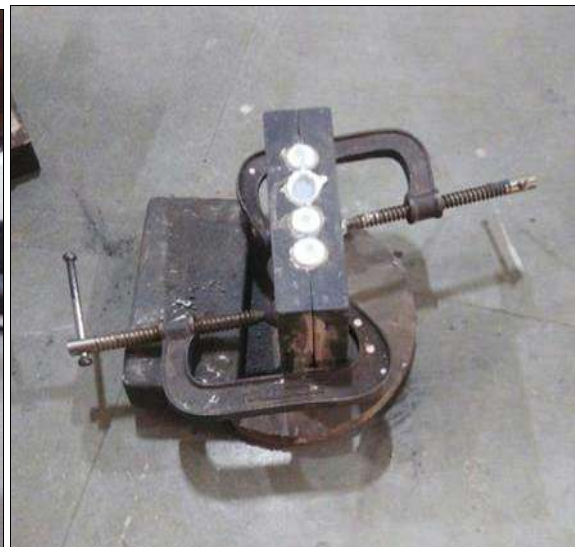
Fig 11: Mould box filled with molten metal
