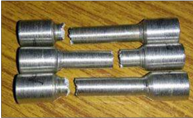
Fig 22: Tensile test broken specimen
