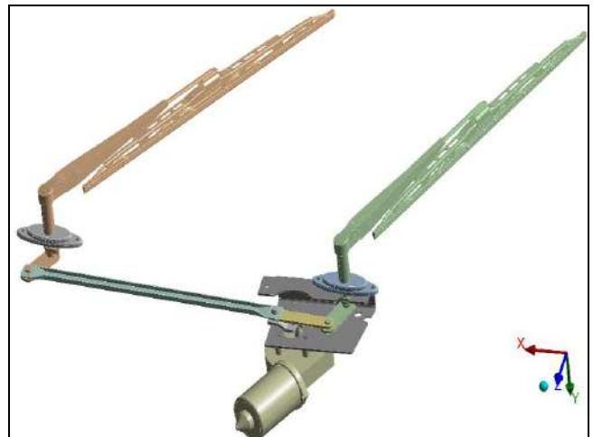
Fig 2: Windshield tandem wiper mechanism
