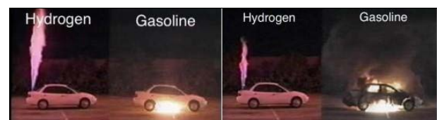
Fig 6: Combustion comparison test of hydrogen fuel cell vehicle and gasoline vehicle (left: 3s; right: 1min)
