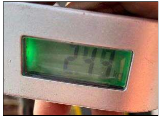
Fig 4: This is a picture of how much force is used to push the lever up 2.49 kgs.
