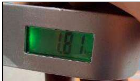
Fig 5: This is a picture of how much force is used to pull the lever down 1.81 Kgs.
